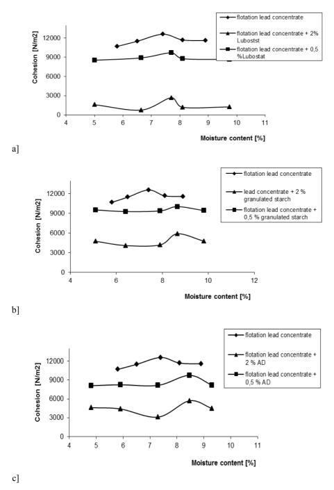
Figure. 1. The changes of cohesion as a function of moisture content: a) flotation lead concentrate + Lubostat; b) flotation lead concentrate+ granulated starch; c) flotation lead concentrate+ AD.
